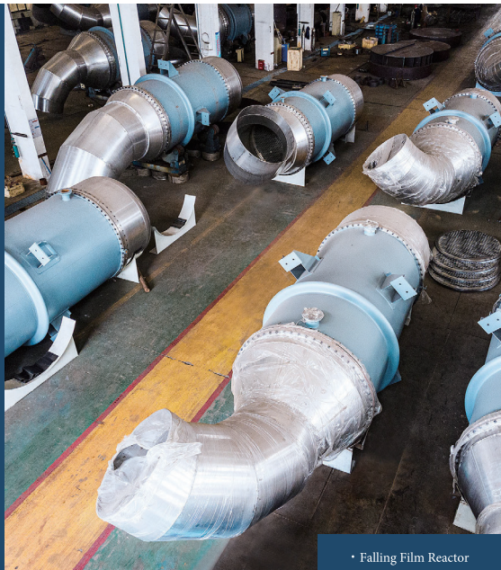
• Falling Film Reactor
